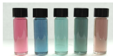
Figure 1: Gold nanorods in aqueous solution. The pink solution on the left are spheres and as you go from left to right the length of the rods increase as the
